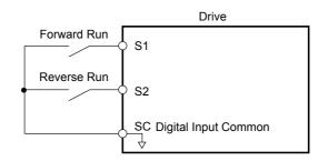
Figure 4.10 Example Wiring Diagram for 2-Wire Sequence
