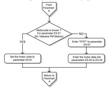
Figure 4.5 Operation with Permanent Magnet Motors
