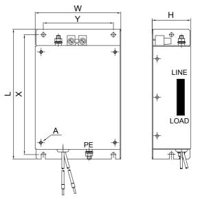
Figure 8.4 EMC Filter Dimensions
