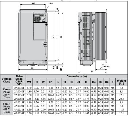
Table 2.6 IP20/NEMA Type 1 (without an EMC filter)
