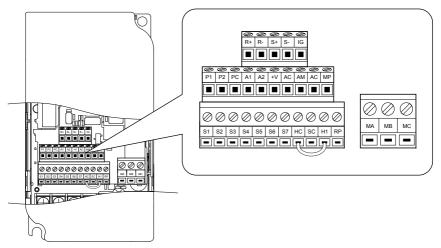
Figure 3.5 Removable Control Circuit Terminal Block (CIMR-VADDDDDD; CIMR-VUDDDDDD)
