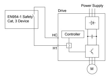
Figure 8.7 Safe Disable Wiring Example
