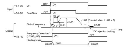
Figure 4.7 Holding Brake Time Chart
