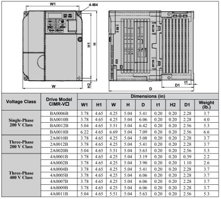
Table 2.3 IP20/Open-Chassis (without an EMC filter)
