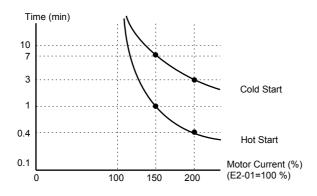
Figure 8.6 Motor Overload Protection Time
