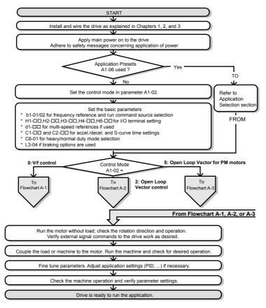
Figure 4.2 Basic Start-Up and Motor Tuning
