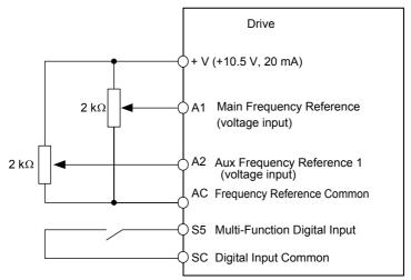
Figure 4.9 Switching between Main/Auxiliary Frequency References
